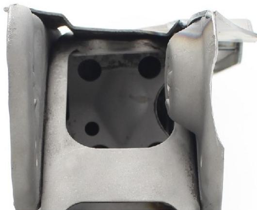
27. Remove spatter and sharp edges. Apply appropriate coating.
