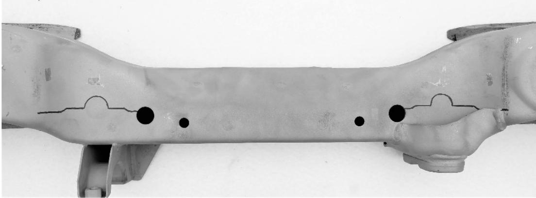
8. Position Template\_7 as shown in the picture. Mark the cutting line.
