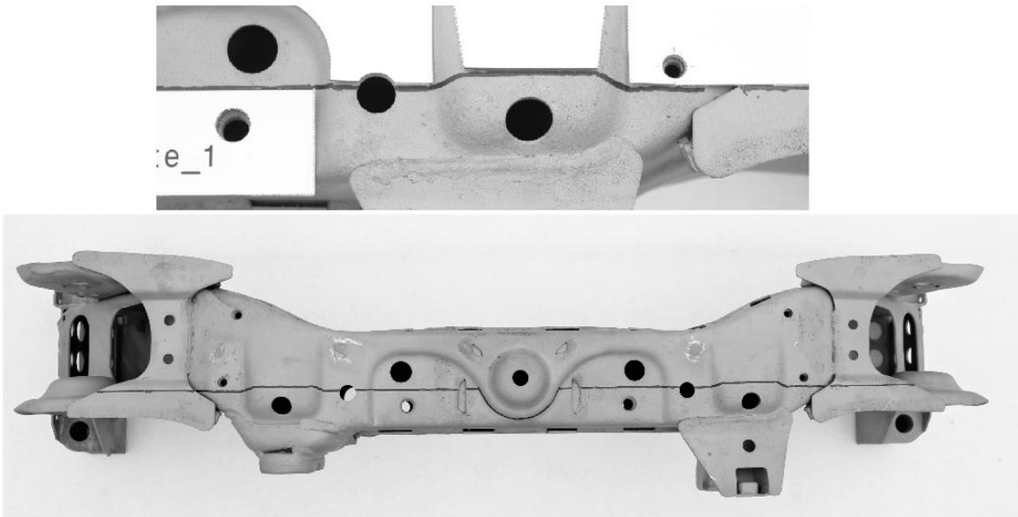
7. Turn the subframe over and position Template\_3 and Template\_4 as shown in picture. Mark the cutting lines. If possible, mark the centre of the arc and drill with a 25mm/1" drill bit. If not, cut it out later with the angle grinder.
