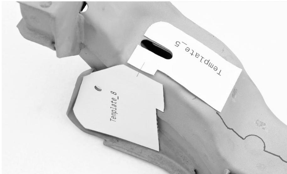
11. Extend the cutting line to the end of the subframe.
