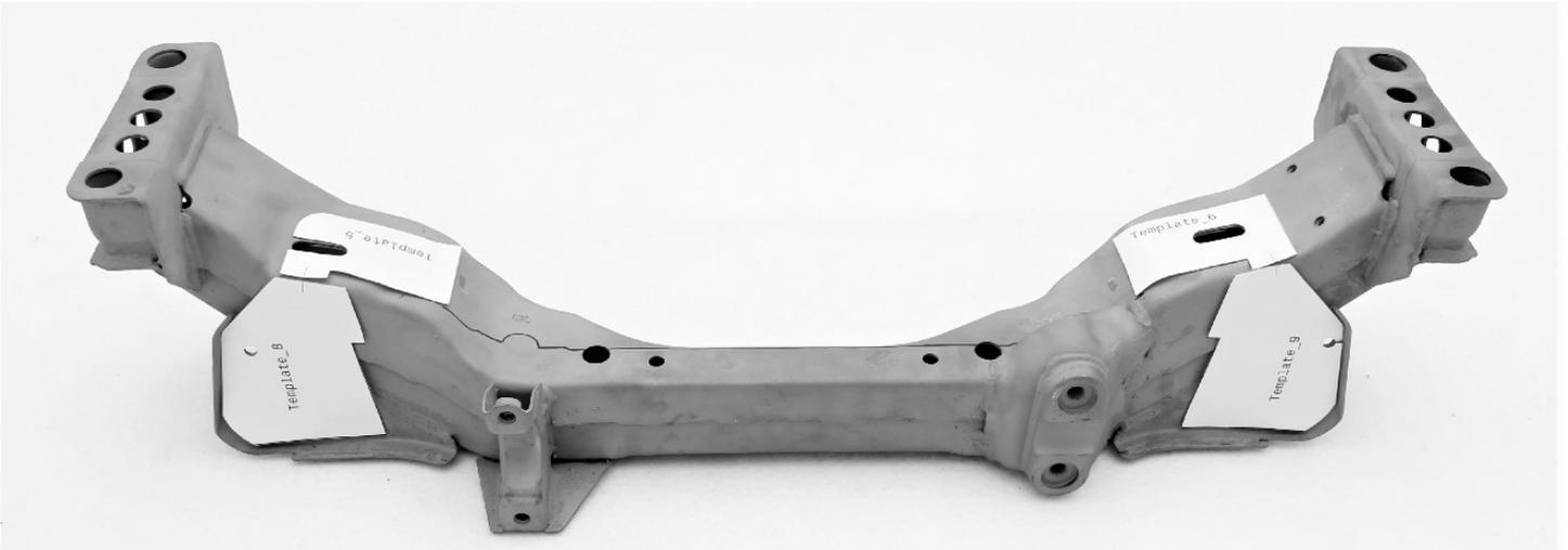
10. Make sure the dotted lines on the templates match each other and mark the cutting line.
