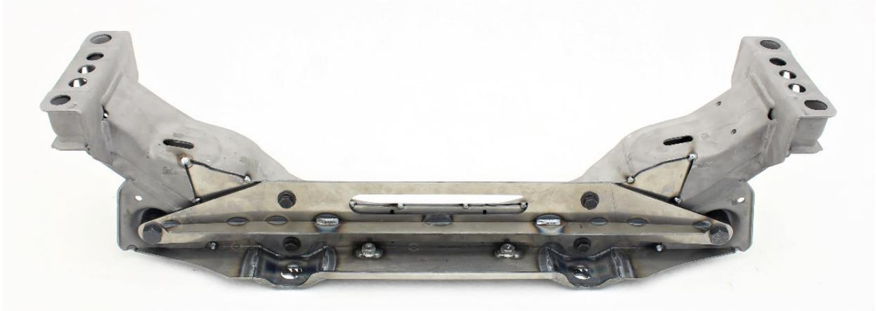
20. Keep the jig in place and fully weld the insert where possible. For extra support, You may temporarily connect the subframe mounts, e.g. with a tube or angle iron. Tube length is approximately 750mm.
