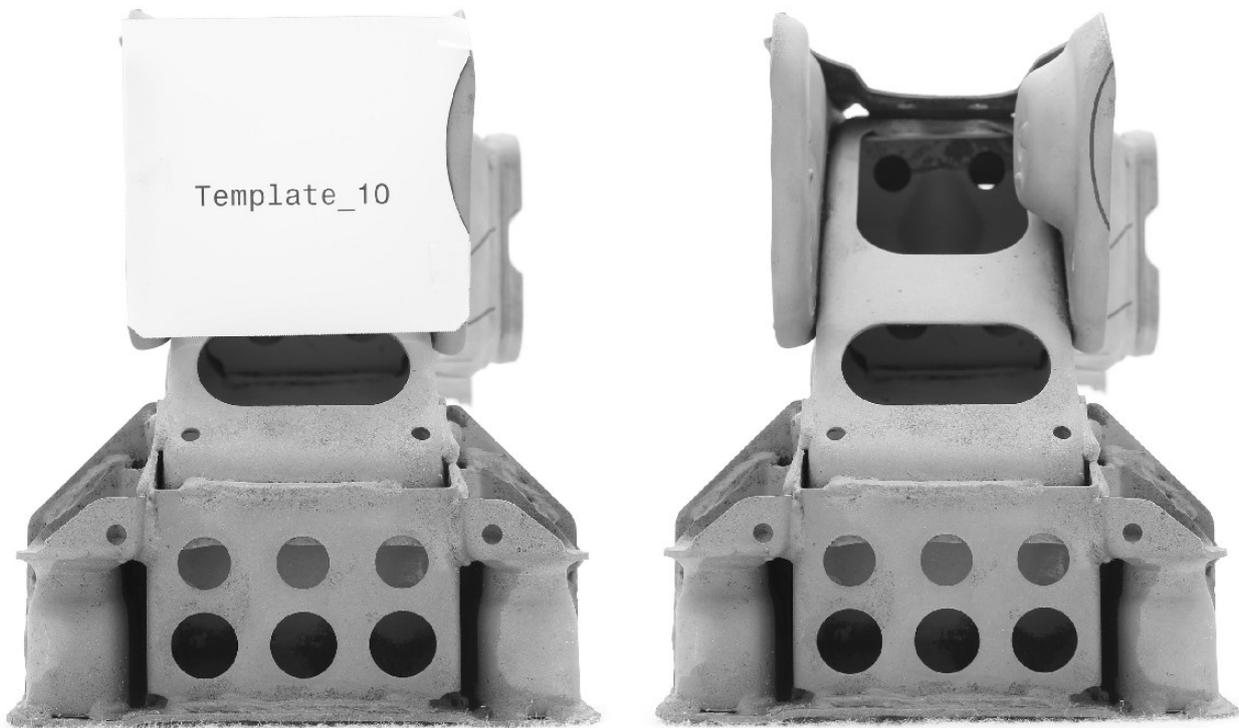
26. Cut the marked section and smooth out any sharp corners. Do this only after welding the subframe.
