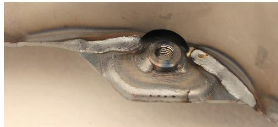
22. If possible, weld the inner walls to the relocation insert from the inside.
