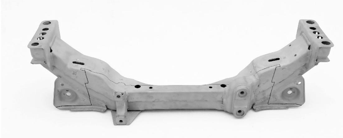
13. Cut the marked lines and remove the sections highlighted in the picture.
