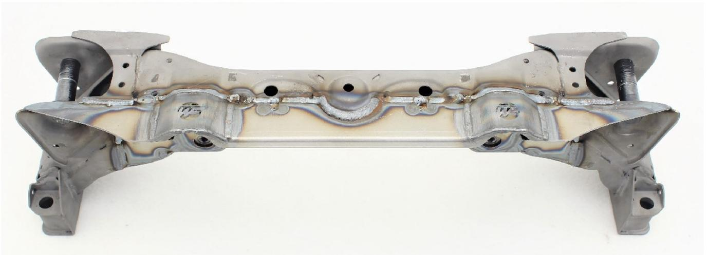
24. Grind down the welds from the subframe brace mounting area.
