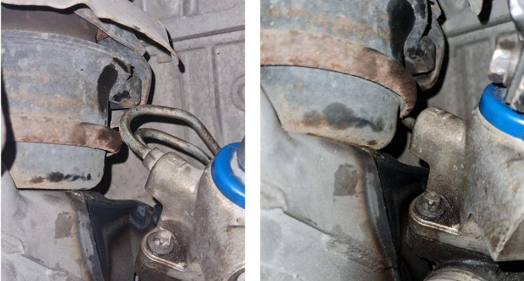
32. Before installing the rack extender spacer, clean the threads inside the rack. After cleaning use thread lock on the spacer. Hold the rack shaft end with a spanner while torquing the spacer.
