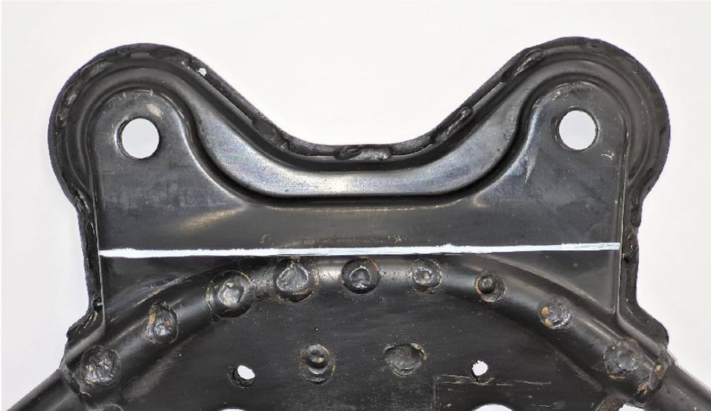
36. To install [Wisefab Nissan 350Z Front Drift Angle Lock Kit](#), the little tabs inside the control arm mounts need to be ground off or pressed flat.
