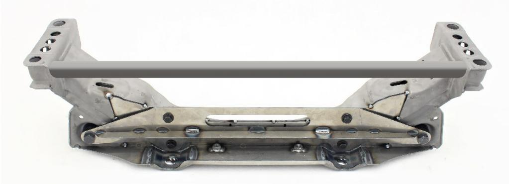
21. DO NOT weld to the threaded bushings. Clearance for the bolts must remain.
