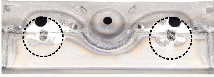
25. Position Template\_10 as shown in the picture. Mark the cutting line. Template\_10 is symmetrical and could be used on both sides of the subframe. The positioning and marking can be done before any cutting or welding.
