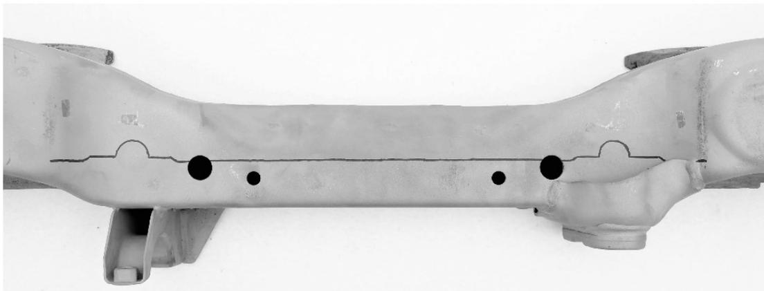
9. Position Template\_5 and Template\_8 on the left and Template\_6 and Template\_9 to the right as shown in the picture.
