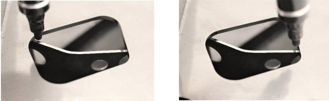
17. Draw an arc from these two points approximately 12mm/ 0.5" deep. Remove the marked section. For LHD cars do this modification to the left side. For RHD cars, to the right.
