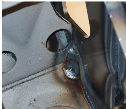
23. Remove the welding jig but keep the long dummy bushings in place. Weld all the areas that were obstructed by the jig. Also bend and weld the control arm mount gusset. Avoid overheating the parts to minimize distortions.
