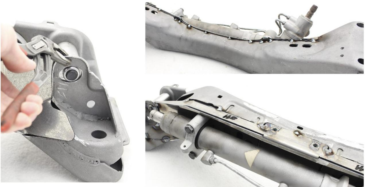
22. Completely weld the insert to the subframe. We recommend to keep the steering rack mounted when welding but make sure that the plastic steering rack bushing won't melt. Avoid overheating the subframe and the rack relocation insert to minimize distortions.
