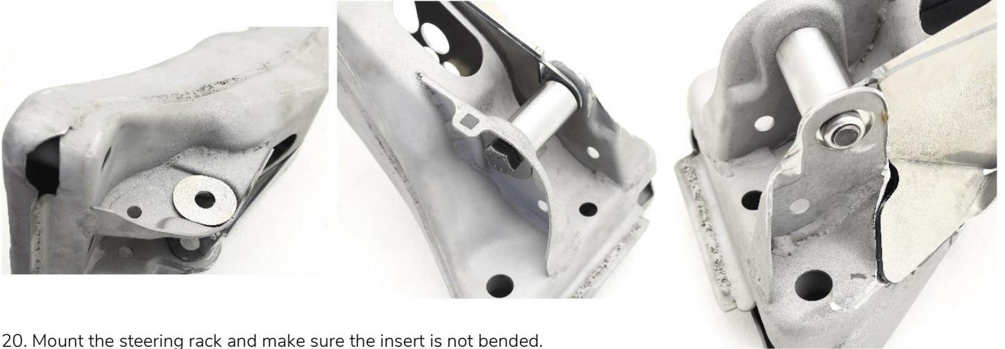
20. Mount the steering rack and make sure the insert is not bended.
