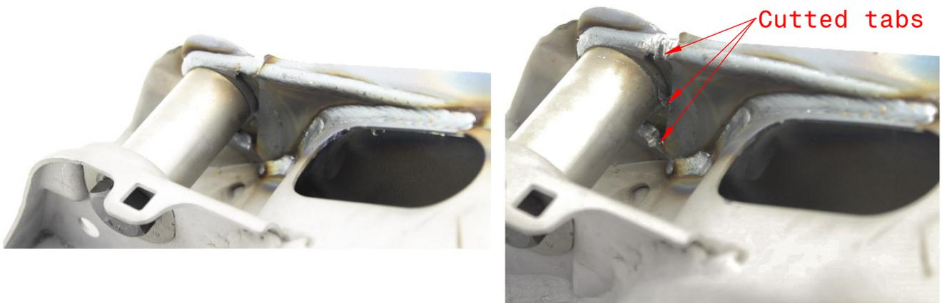
25. Remove all the bolts and washers. Remove any weld spatter and sharp edges. Apply appropriate coating.
