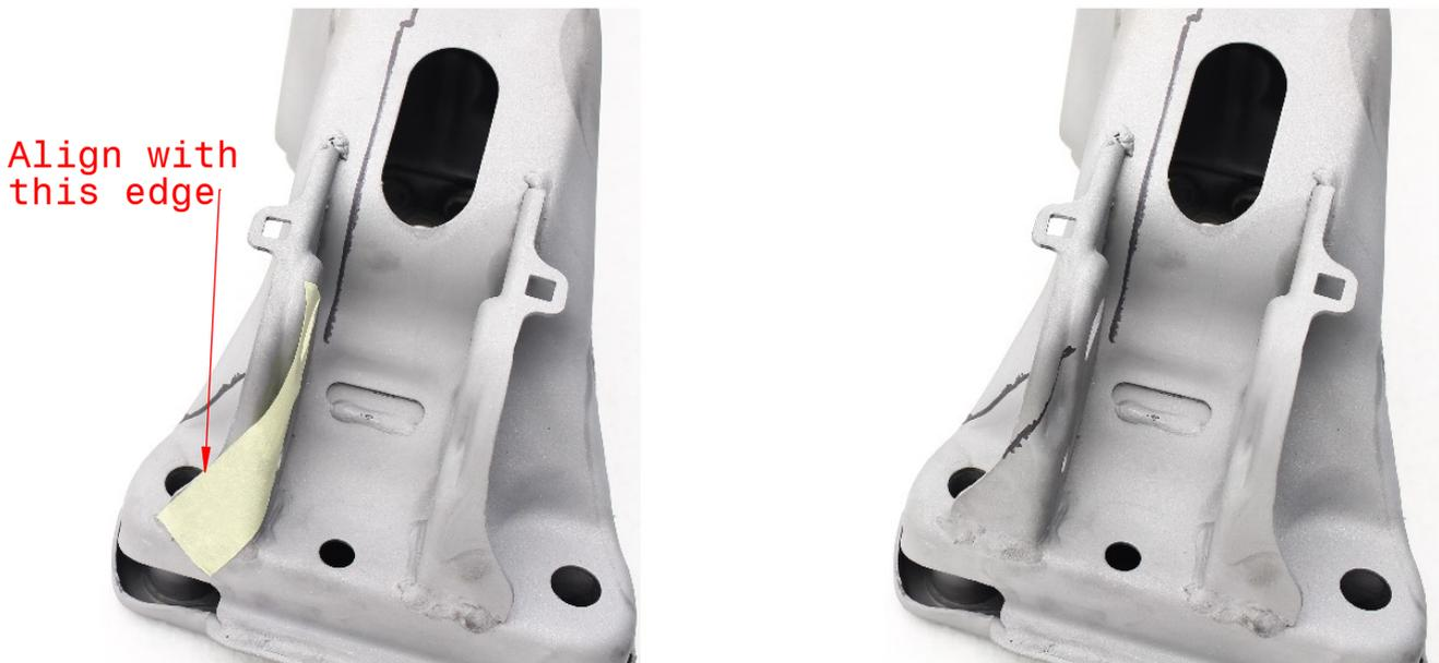
13. Hatch the area as shown on picture. Keep the mounting surface. Repeat the same on the other side.
