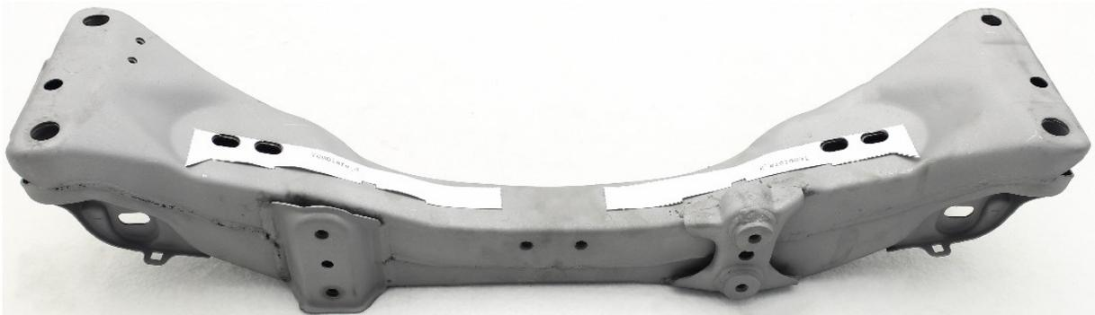
9. Connect the templates with the masking tape (along the cutting edge) and mark the cutting lines.
