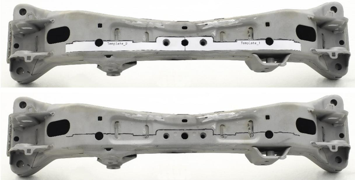
7. Place the masking tape along the cutting edge and cut the tape as shown in the picture. Check with the washer WFIS9\_106 if there are at least 3 mm gap between the mounting surface and the masking tape edge. Repeat the same on the other side. Mark the cutting lines.
