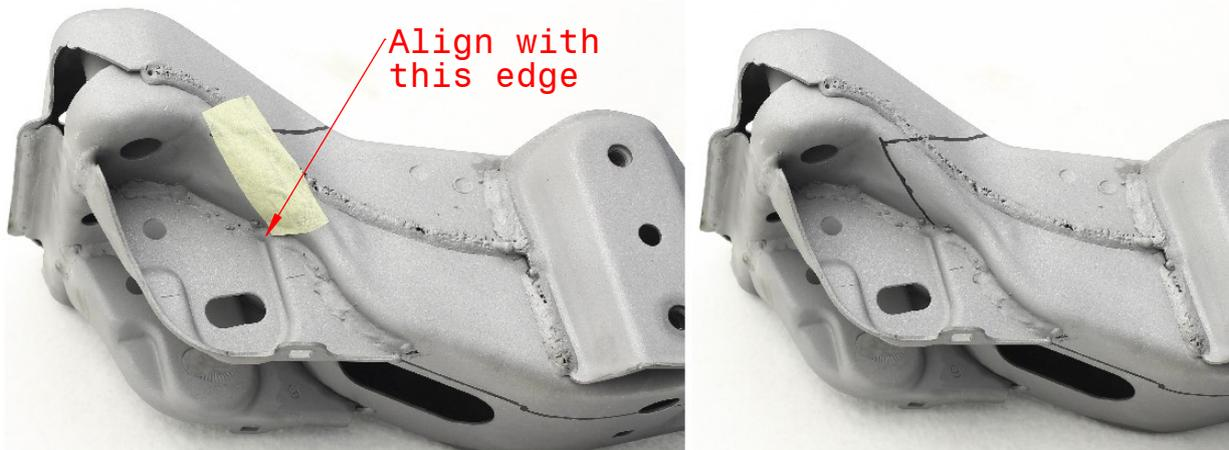
12. Place the masking tape along the edge to the mounting surface. Mark the cutting line.
