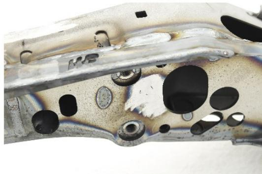
24. If the steering rack relocation needs to be Formula Drift legal, the tabs between the insert and lower control arm mount needs to be cut through. Use chisel to cut the tabs. NB! If the subframe does not have to be FD legal, then this is not necessary.
