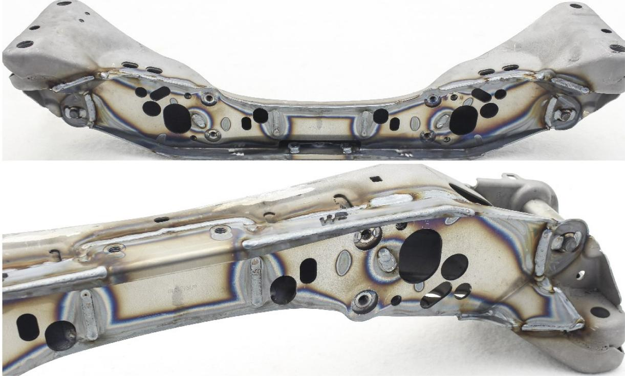
23. Grind flat the weld next to the steering rack mount.
