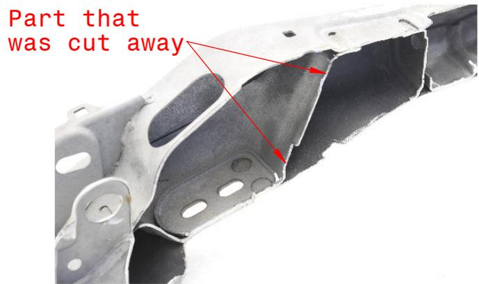
18. Place the steering rack relocation insert to the subframe. Please check that insert is not interfering with subframe or the insert itself is not bent. Check if there are enough room behind the steering rack mounting nuts to mount the bolts.
