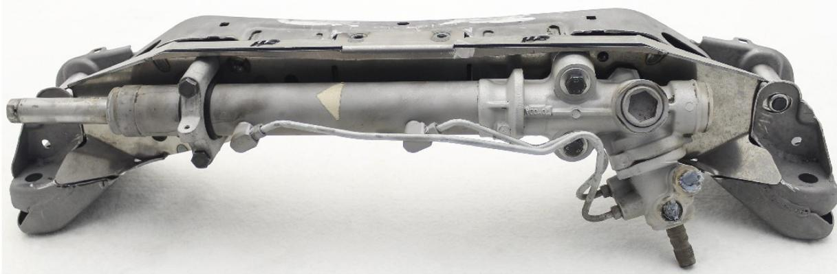
21. Tack weld the relocation insert. If the stock control arm mount is away from the rack relocation surface then clamp them together while tack welding.
