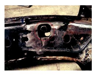
Seamweld the fasteners and cut off the rest of the material including the holes for template fixing.
