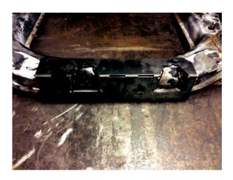
Note: Mark the lower edge of the cut out according to the sharper angle of the template side
