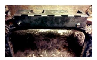
Using the template mark the holes of the cut outs and clearance holes underneath.
