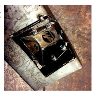
Point weld the fasteners and remove the template. **Note:** grind town the template point welds to be able to remove the template.
