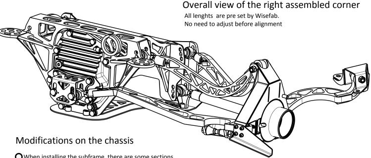
Owhen installing the subframe, there are some sections that need to be cutted on the chassis near the front mounting points of the subframe.
