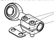
Loosen the two bolts to adjust caster
