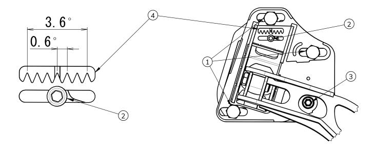
When removing the knuckle for repairs, keep the M6 allen bolt (2) tightened to avoid changing the toe setting.
