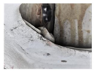
9. For maximum toe-out on E36 body, the inner sill panel needs to be cut or stretched at the area shown in the picture.
