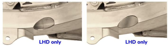
8. Cut off the marked section from the original steering rack mounts as seen in the picture. Grind the surface flat. Also grind/sand clean any surfaces which are about to be welded.
