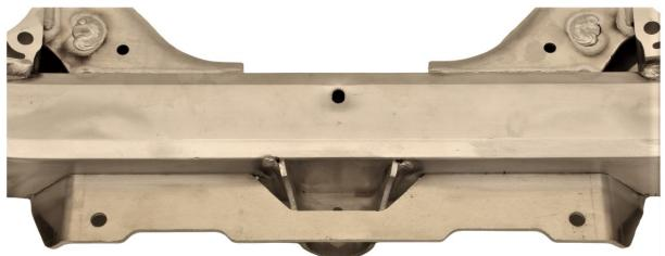
12. Use the E90 steering rack to locate the new upper rack mounts. Make sure the steering rack is level with the subframe. Tack weld the new mounts.
