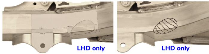
7. Cut off the marked section. The area could also be carefully hammered in.
