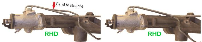
4. On the **LHD** rack, one line needs slightly re-routing as shown in the pictures. Make sure not to kink the line while bending and unbending.
