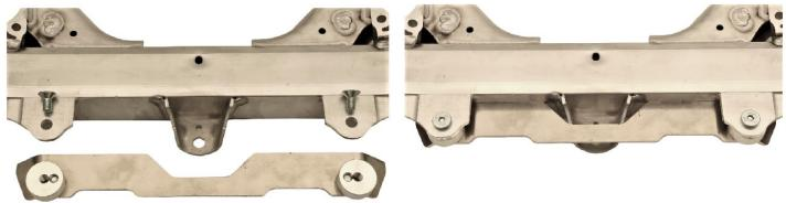
10. Weld the new mount to the subframe. Weld from the underside of the mount.
