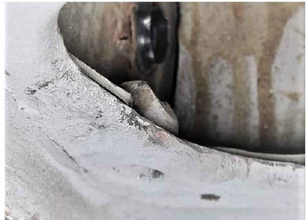
6. For maximum toe-out on E36 body, the inner sill panel needs to be cut or stretched at the area shown in the picture.
