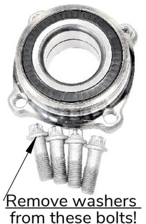
With Wisefab halfshaft use the outer ABS mounting without spacer
