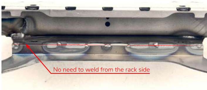
Make sure that the strengthening plate (From step 19.) is welded from the inside
