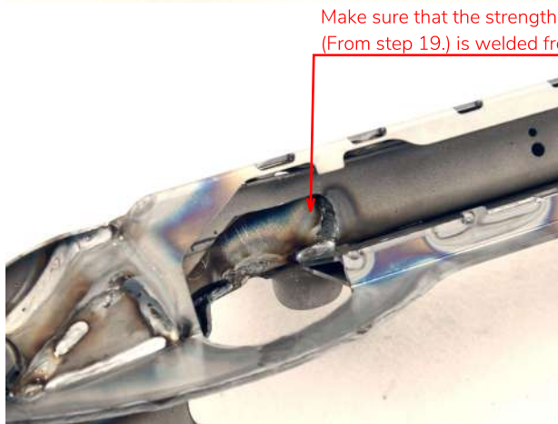
No need to weld from the rack side
