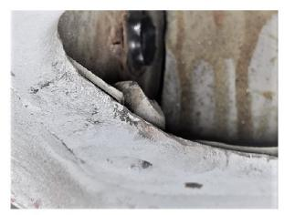
6. For maximum toe-out on E36 body, the inner sill panel needs to be cut or stretched at the area shown in the picture.
