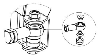
When installing the outer tie rod to the knuckle make sure that the outer tie rod is at the up most position and the supplied bushing is below it.
