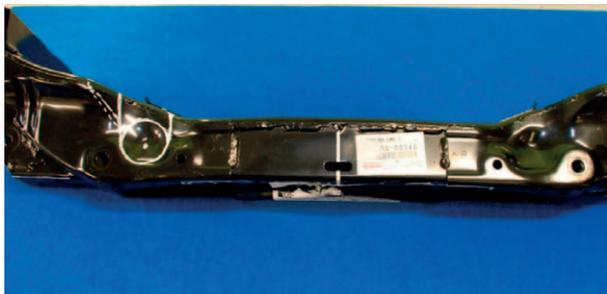
Remove the threaded tubes used for fixing the original steering rack.
