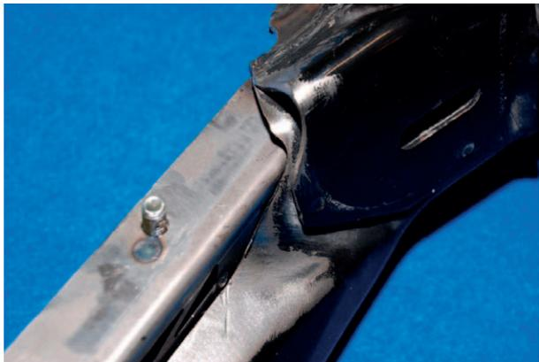
Weld the steering rack fastener
