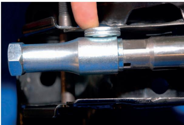
Use spacer to position the steering rack vertically. Position the spacer between 12 mm A-arm polt and steering rack extender cylindrical section. Correct spacer thickness is 23mm.
