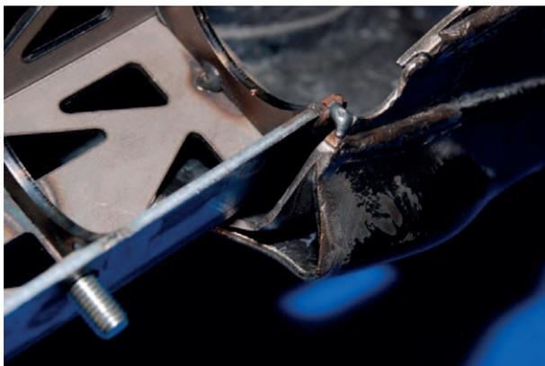
Using cutting, bending and welding make enough clearance for the steering column extender and its fixing bolt (shown with the red circle on the picture right).
