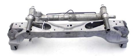
16. Box in the subframe near the steering shaft and tack weld the plates in place
