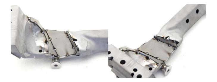
17. Use the circular part of the plate to fill the hole in the subframe
