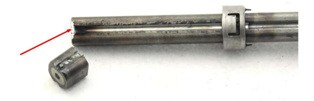
9. Clean all the parts and assemble. Use bearing grease between the sliding element. If the locking cap does not have groov to lock on to then tack weld it place
