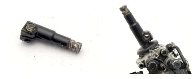
2. If the steering shaft is to long and can not be fitted with the OEM steering shaft extender then it can be installed without it.
