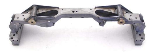
20. Test fit the steering rack to the subframe. If everything is fine then apply the appropriate coating (Black powder coating in the picture)
