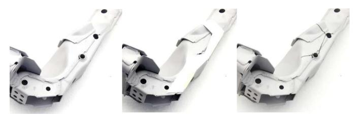
9. Position the Template 4 as shown on picture. Mark the cutting lines. Mark only the side were the steering shaft is. Right side for RHD and left side for LHD
