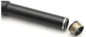
7. Test fit the inner side of the steering shaft with the shortened part. If the dimension A (that was previously measured) can be achieved and there is room for the inner side to slide in extra 40 mm, then the inner side can be left uncut. If it can not move in the extra 40 mm then it needs to be shortened. For example if it goes in only about 25 mm from the A dimension then the inner part has to be shortened by 15 mm.
