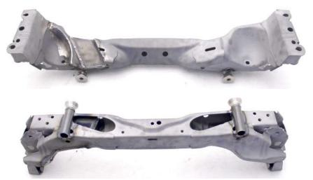
20. Add the strengthening plates. First tack weld and then seam weld them in place. DO NOT REMOVE THE STEERING RACK WHILE WELDING. Avoid overheating the parts to minimize distortions. Remove the spatter and sharp edges after welding.
