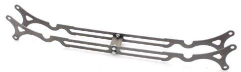
13. Bolt on the welding jig (using the OEM lower control arm bolt), new steering rack mounts and the steering rack to the subframe. Use the WFGD3\_116 washers between the jig and subframe to space the jig away from the subframe. Then clamp the middel plate (plate between the 4 bolts) on the jig so there are no gaps between and tack weld it to the jig.
