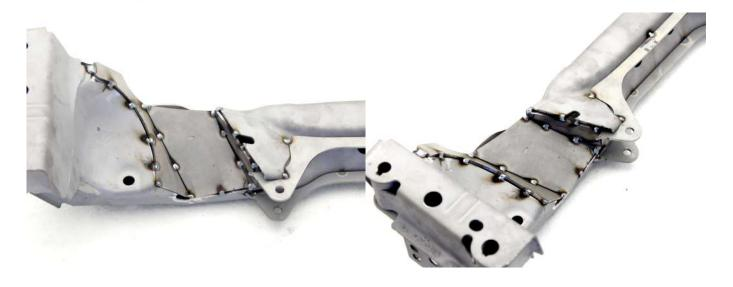
16. Use the circular part of the plate to fill the hole in the subframe
