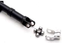
3. Remove the two bearing cups from the universal joint. Insert the universal joint cross with pre fitted Wisefab universal joint housing in the steering shaft universal joint housing and press in the two bearing caps. After the two bearing caps are pressed in fix them by hitting the top part of the universal joint housing with a chisel.
