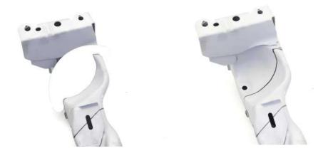
10. If the OEM engine mounting points on the subframe are not use then remove them from the subframe. If they are still needed then use the WF8691\_101 to mark the cutting lines. Both engine mounts has to be marked.
