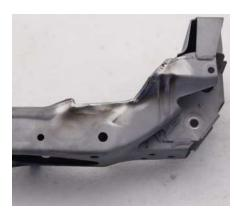
19. Test fit the steering rack to the subframe. If everything is fine then apply the appropriate coating (Black powder coating in the picture)
