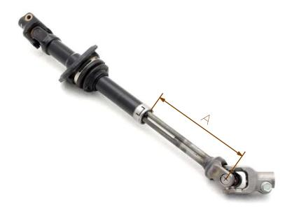
5. The OEM steering shaft is expandable. To shorten the shaft the extended part has to be shorten. First take of the cap.
