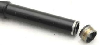
8. Test fit the inner side of the steering shaft with the shortened part. If the dimension A (that was previously measured) can be achieved and there is room for the inner side to slide in extra 40 mm, then the inner side can be left uncut. If it can not move in the extra 40 mm then it needs to be shortened. For example if it goes in only about 25 mm from the A dimension then the inner part has to be shortened by 15 mm.
