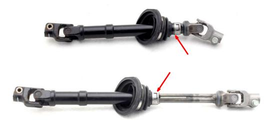
6. Pull the steering shaft apart. Do not lose any of the bearing balls.
