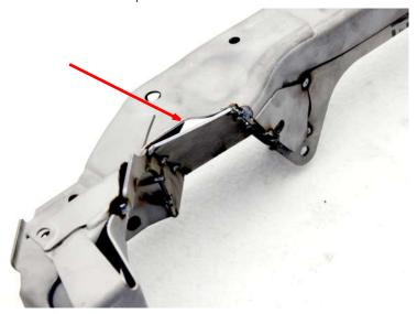
18. Weld all the edges. DO NOT REMOVE THE STEERING RACK OR THE JIG WHILE WELDING. Avoid overheating the parts to minimize distortions. Remove the spatter and sharp edges after welding.
