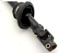
2. Clean the universal joint housing bearing cup surface and make sure there are no sharp edges or score marks.
