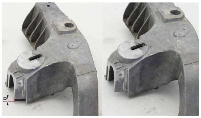
11. Chamfer the sharp edge, same for the other side.
