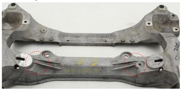
9. Cut off the area between the marked lines
