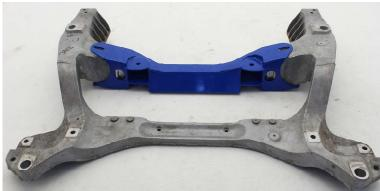
15. Check if it is possible to insert the bolts. If not, use a ratchet strap to align the holes. Make sure everything fits well and there is no interference between the subframe and the steering rack relocation. If the steering rack relocation insert touches the subframe and the holes are still not aligned, use the grinder to grind off the excess material from the subframe.
